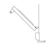
Holding the door at 45°, carefully align the hinge tongues with the hinge slots. Push the door in until you feel the latches locate into position on each side
