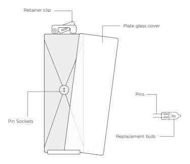
Removing and refitting the oven door
