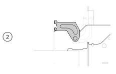
Open the hinge locks fully on both sides
