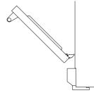
Holding the door on both sides, lift door back up to 45° and carefully pull the door out and away from the hinges.
