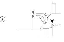
Open the door completely and ensure both hinges are secured by the correct notches.
